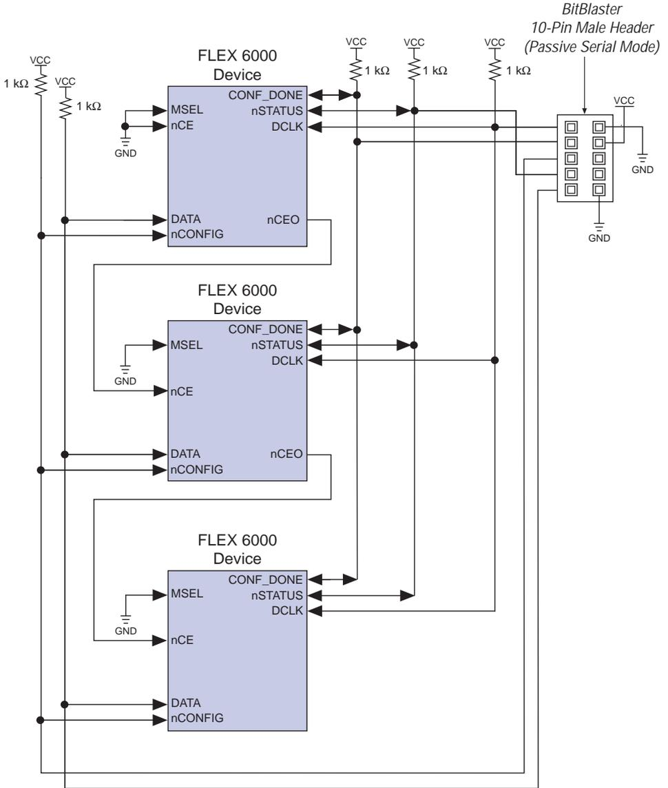
FLEX 10K and FLEX 6000 devices can also be configured in the same configuration chain. The nCEO pin of a FLEX 10K device can be connected to the nCE pin of a FLEX 6000 device and vice versa. The CONF\_DONE and nSTATUS pins of all the devices in the configuration chain must be tied together.
