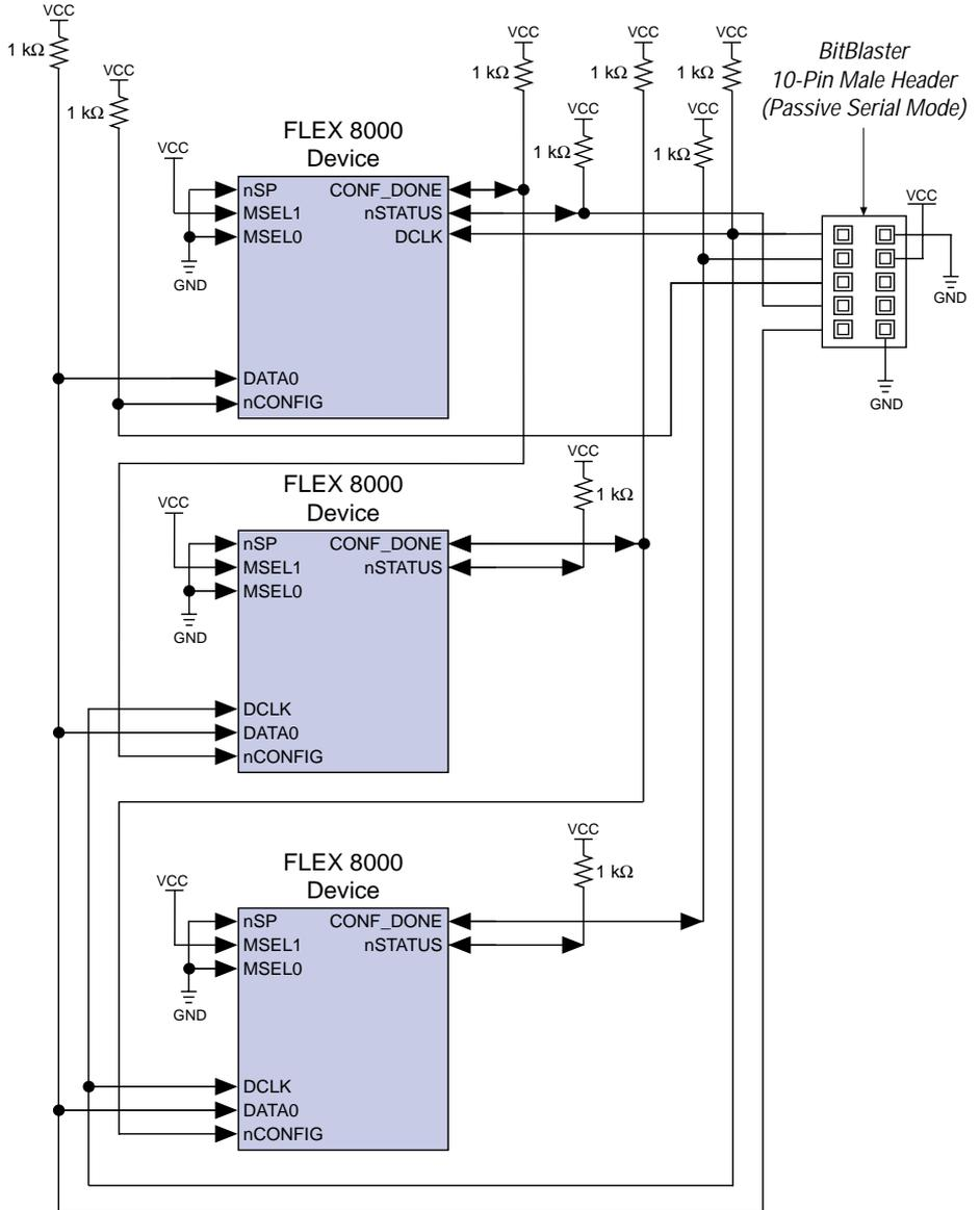
Figure 8. FLEX 6000 Multi-Device Configuration with the BitBlaster Cable
